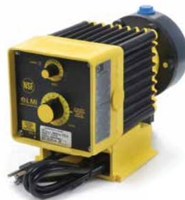
**LMI B SERIES & C SERIES CHEMICAL FEED PUMPS** — Electronic solenoid driven chemical feed pumps with variable speed and stroke length adjustments. Rugged chemical resistant housing for corrosive environments and chemicals. Four Function Valve AutoPrime liquid end allows for de-gassing during pump priming and operation when used with Sodium Hypochlorite (Bleach).
