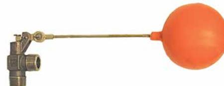
**BRONZE FLOAT VALVES** — Heavy duty bronze float valve with Buna-N disc is rated at 125 psi. Third party certified to NSF/ANSI 372. Tapped for 1/4-20 SAE rod, with threaded outlet. Stainless steel rods and plastic floats ordered separately.
